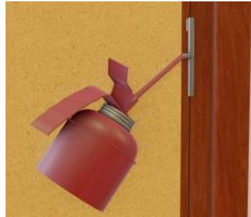
Example of lubrication of hinges.
