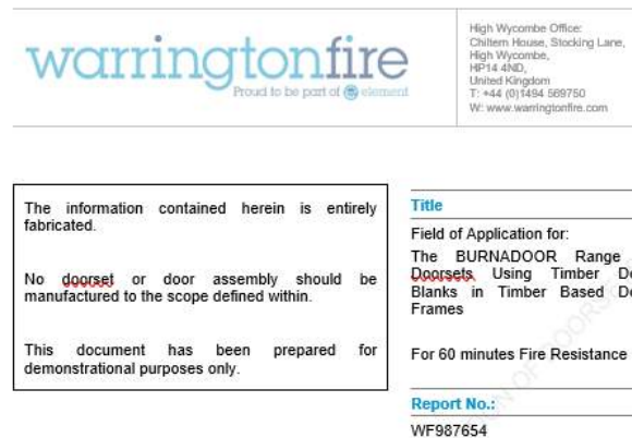
Example of supporting evidence for a doorset design in the form of a field of application.
