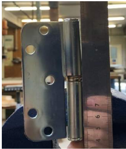
Example of a lift off type hinge where the pin has bent over time.
