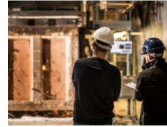
Example of a typical fire resistance test furnace, for when a test may be required.
